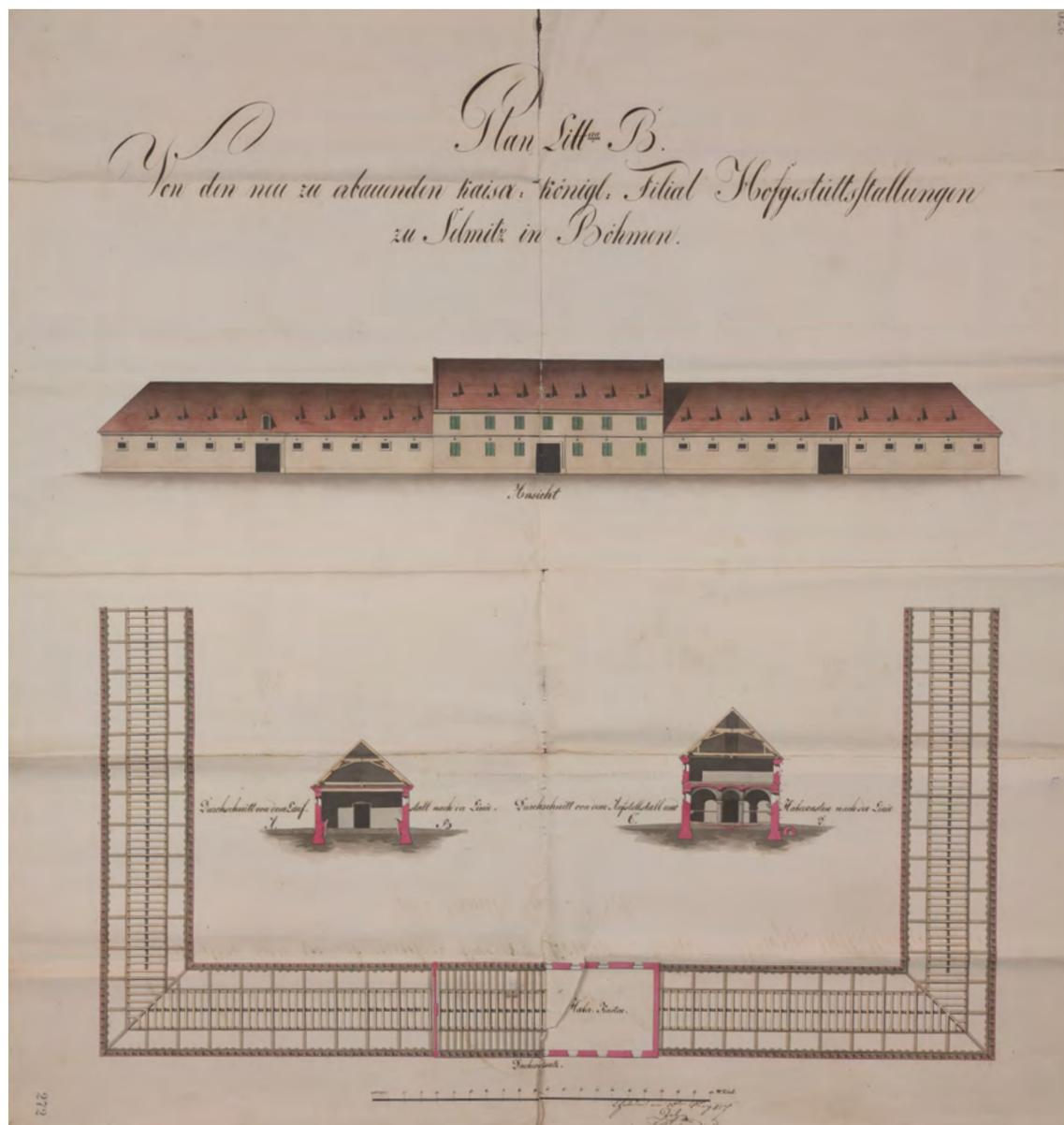
017 Mauritz Jahn's plan of the Františkov farmstead construction from 1828. Floor plan of the granary, trusses above the stables, cross-sections of the buildings and the front facade. An example from the extensive set of archive documents illustrating the Classicist reconstruction of the farmstead. National Archive.
